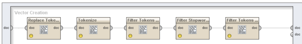
Figure 5: Sub-process of “ Process Documents from Files ” operator Source: Screenshot of RapidMiner Version 6.5, sub-process of “ Process Documents from Files ” operator including the operators “ Replace Tokens ”, “ Tokenize ”, “ Filter Tokens (by Length) ”, “ Filter Stopwords (German) ” and “ Filter Tokens (by POS Tags) ”.
